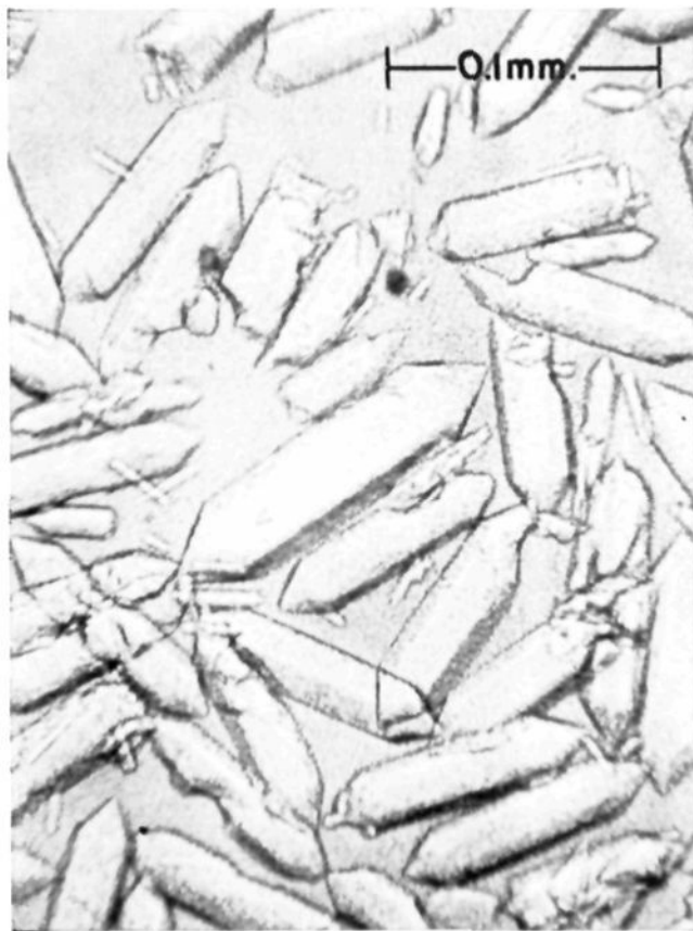
Fig. 3.—Bovine serum albumins crystallized from 0.14 mole fraction ethanol; \Gamma/2 = 0.4 ; pH 5.5; -5^\circ .
